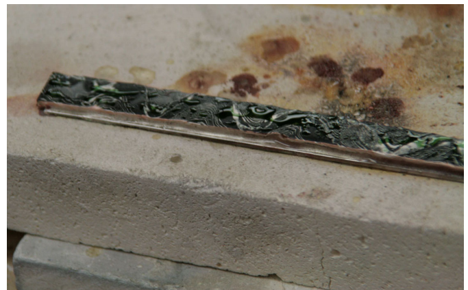
A well soldered joint
